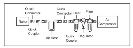
Figure 2. Filter/Lubricator/Regulator Unit.
